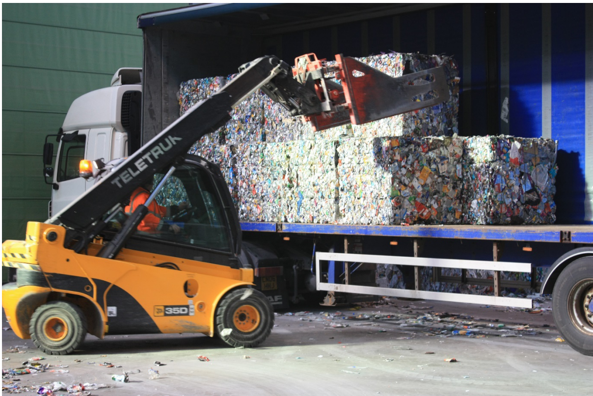
Sorted and baled materials being loaded to be despatched to a reprocessor
